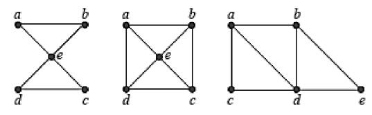
The graph G1 has an Euler circuit, for example, *a, e, c, d, e, b, a*. Neither of the graphs G2 or G3 has an Euler circuit. However, G3 has an Euler path, namely, *a, c, d, e, b, d, a, b*. G2 does not have an Euler path.
